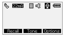
Figure 3. LCD Display Screen
