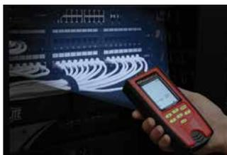
Easy to read, backlit LCD screen with large icons, glow-in-the-dark keypad, and built-in LED flashlight for use in dark areas.
