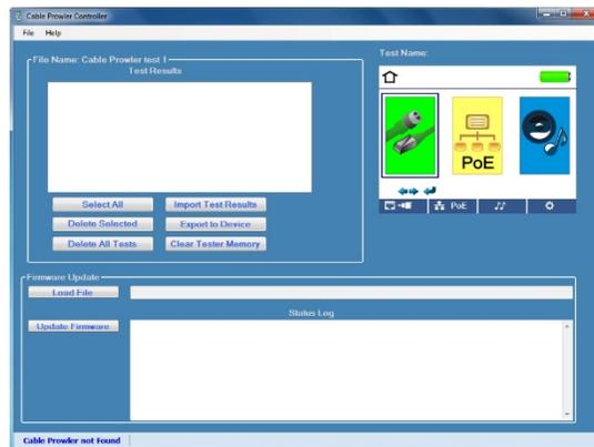
3. Click on "Import Test Results" to upload test results from the Cable Prowler to the Cable Prowler Application
